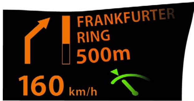
HUD image showing distortion for improper installation or adjustment
